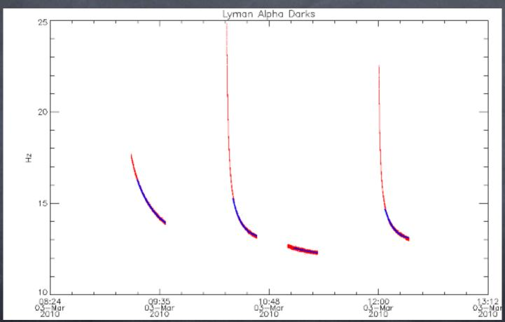
The red data points are the dark current measurements. The blue curve is the model fit used to remove the effect of stabilization.
