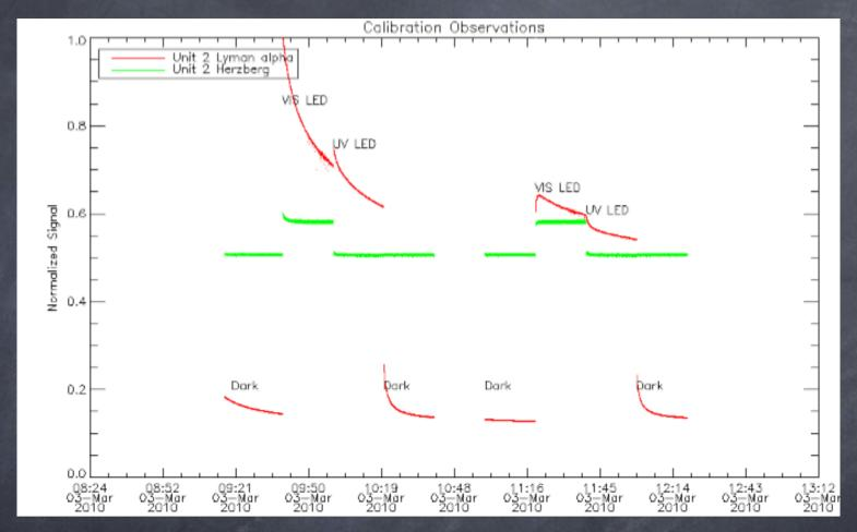
This plot shows the standard calibration observing sequence. The dark current is measured for 20 minutes, then the VIS LED is switched on for 20 minutes, then the UV LED, and finally another 20 minutes of dark current. The sequence is then repeated.
