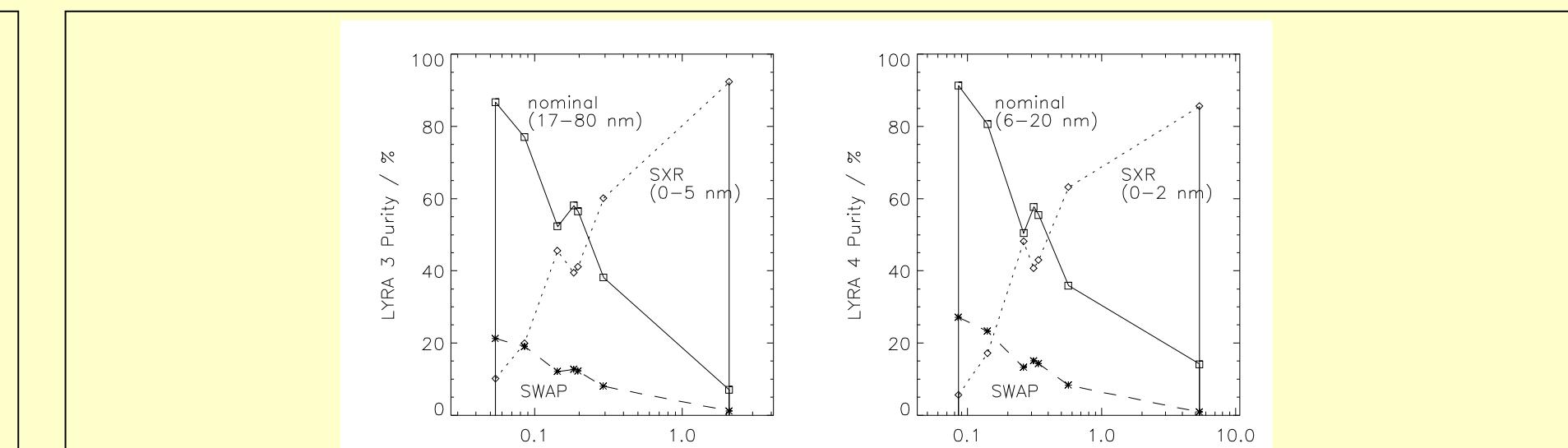
From LYRA's short-wavelength channels 3 and 4, the SWAP signal can be estimated as a subset of both the nominal signals; the SXR signals (0-5 nm and 0-2 nm) can be estimated as the complement of the nominal signals.
