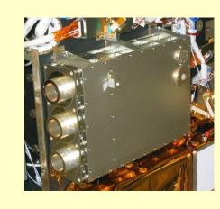
SWAP is a small EUV telescope that will image the solar corona at a temperature of 1 million degrees K. SWAP will continue the systematic CME watch program of SOHO/EIT at an improved cadence and monitor events in the lower solar corona that might be relevant for space weather
