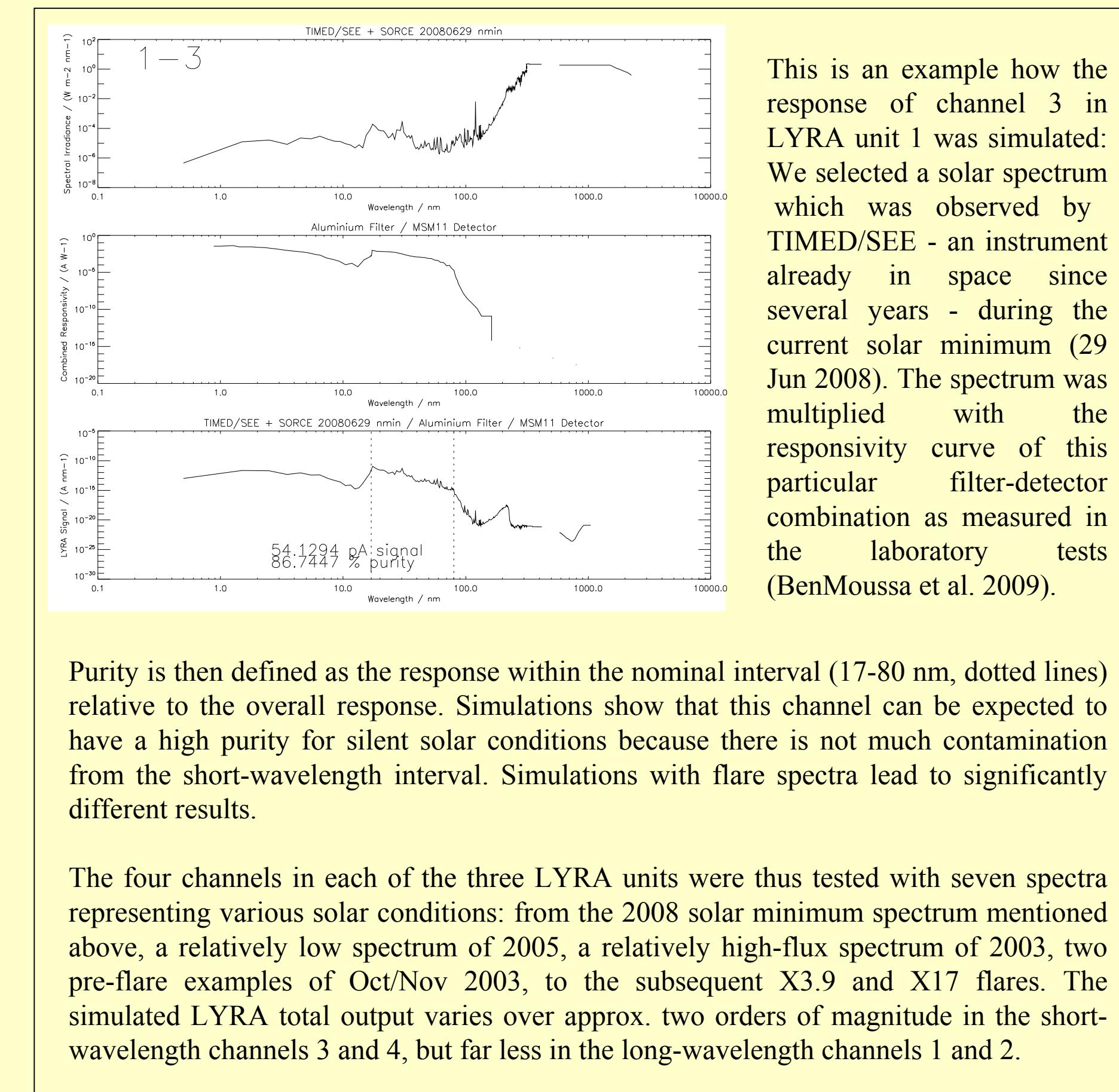
This is an example how the response of channel 3 in LYRA unit 1 was simulated: We selected a solar spectrum which was observed by TIMED/SEE - an instrument already in space since several years - during the current solar minimum (29 Jun 2008). The spectrum was multiplied with the responsivity curve of this particular filter-detector combination as measured in the laboratory tests (BenMoussa et al. 2009).
