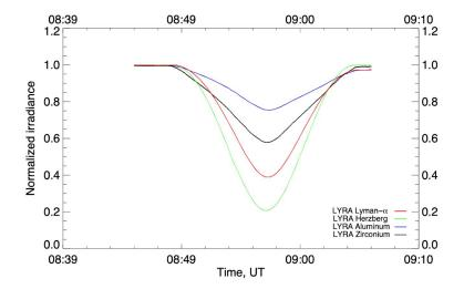
The two occultations were also observed by LYRA's "calibration unit" (unit 1) in addition to the nominal one (unit 2). The plots above show normalized observations by LYRA during the two passes in the eclipse zone. The colors correspond to the observations by the four channels of LYRA: red = Lyman-alpha, green = Herzberg, blue = Aluminum, black = Zirconium.
