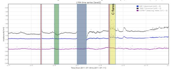
The calibration campaign is annotated in blue, the back-up acmpaign in green, and data gaps due to propulsion campaigns in red. The peaks in LYRA signals are due to solar flares. The tiny, periodical peaks in SWAVINT were caused by crossing over the SAA.
