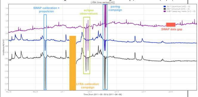
The calibration campaigns are annotated in blue and orange, a SWAP data gap in red. The eclipse observations are shown in green. All those campaigns are described below. The peaks in LYRA signals are due to flares, the little, periodical peaks in SWAVINT are due to SAA.
