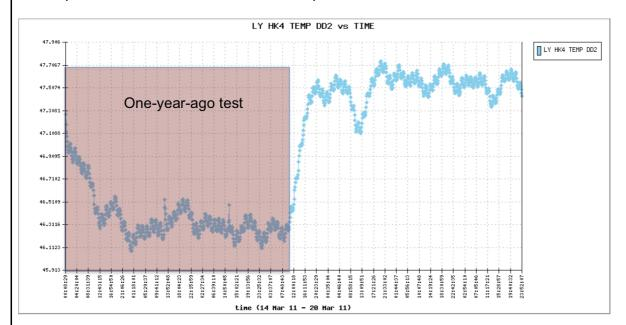
The conclusion of the test is that LYRA temperatures have all globally increased by 3.5 - 4 °C
