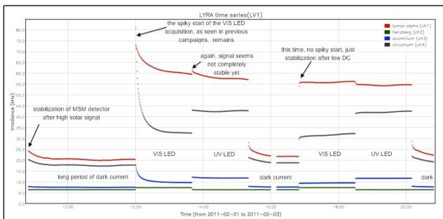
Unit 1 (also mainly MSM) does not see this slowly decreasing signal throughout the LED signals, but also did not acquire solar signal prior to the calibration. Unit 3 does not show any stabilization at all (as expected with Si detectors), just a little peak of 2-3 minutes at the time a LED switches on.
