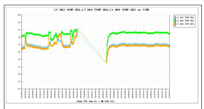
The temperature is still very close to the onboard safety limit of 50 degrees. We expect however that the temperatures will decrease soon as the distance Earth-Sun is increasing again.
