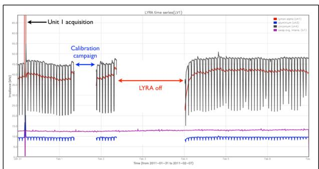
As clear from the figure, no important flares (>B type) were recorded. LYRA was off for 1,5 day due to the hot temperatures onboard (see Sect. 2). The other gap on Feb 1st was due to a calibration campaign (also in Sect. 2).
