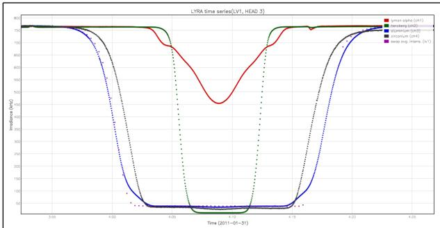
Part of the SWAP average intensities (purple dots) during sunrise are missing in this figure because of a LAR. These images have to be processed in a non-standard way to complete the curve. Analysis is ongoing.
