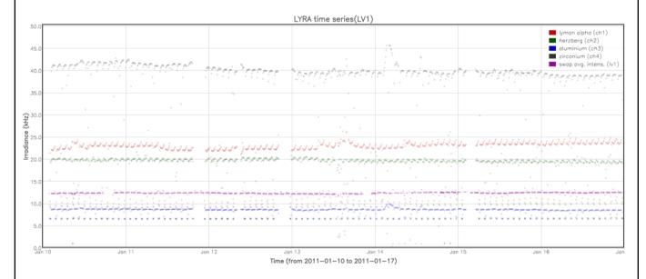
There was no significant jump in Herzberg channel (only small jumps correlated to the opening/cloosing of cover 3).
