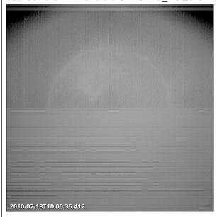
During the first run, the instrument was operated in CORRELATED\_DOUBLE\_SAMPLING. Some images seems incorrect. During the second run, the instrument was operated in DOUBLE\_SAMPLING mode, and the effect similar to the upper shown image can be observed for all delta times. This needs further investigations.
