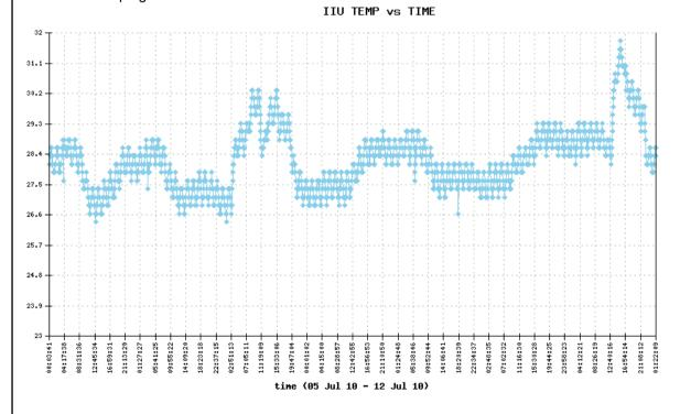
SWAP detector temperature remained fix during the week, increasing slightly during the weekend, presumably due to the parallel campaigns of other instruments .
